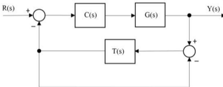
$$\text{Con } G(s) = \frac{1}{s+2} \quad T(s) = \frac{2}{s} \quad C(s)=K$$
